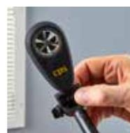
Thumbwheel for attaching/removing threaded universal end
