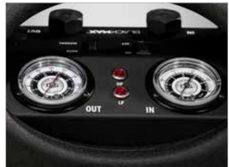
Large 2-1/4" diameter gauges and indicator lights for high pressure or low pressure status
